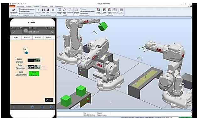
Fig 5. Programming ABB Robots using the ABB RobotStudio IDE.
