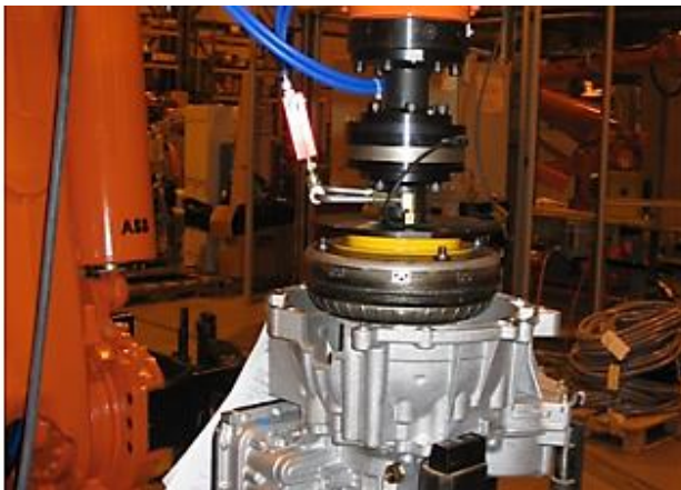
Fig 9. Torque converter installation example utilizing force-controlled assembly.
