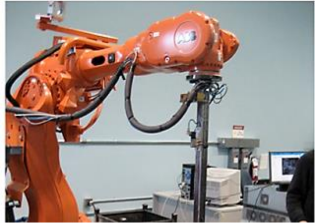
Fig 8. This is an example of a test installation for automatic bin selection. Here, the gripper is mounted on a lengthy beam so it may access all things in the deep bin without touching the walls of the bin or approaching singularities.
