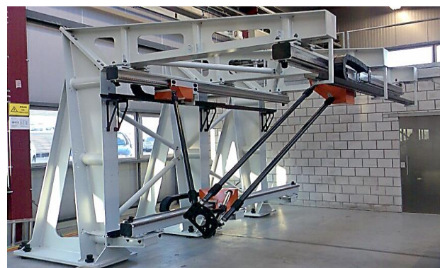
Fig 6. A Gantry-Tau prototype as part of the SMERobot TM Initiative.
