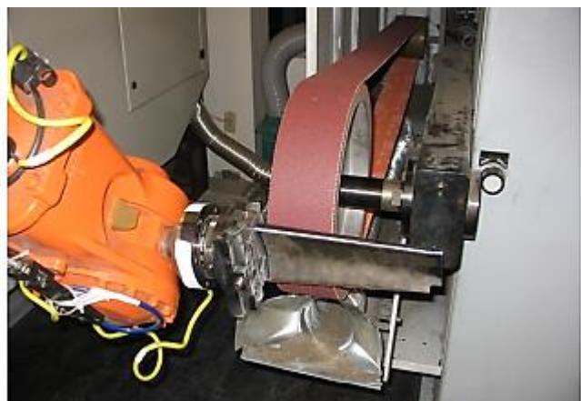
Fig 10. Installation of a turbine employing force-controlled grinding as an example.
