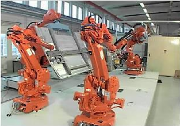
Fig 7. The ABB MultiMove concept is used to operate four cooperative robots. The task is carried out by one robot while three others carry out separate operations on it in a coordinated manner.
