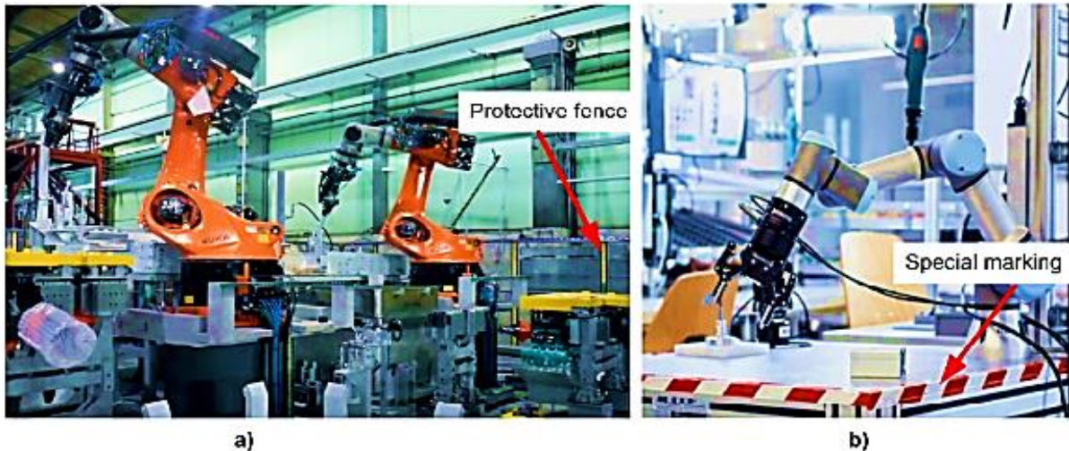
Fig 2. An Analysis of the Differences between the Working Conditions of (a) Industrial Robots and (b) Collaborative Robots.
