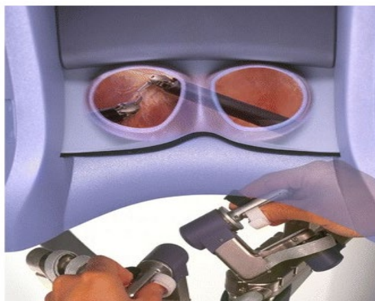
Fig 2. Application of grips that are perpendicular to the binocular viewers' optical axis.
