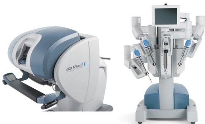
Fig 1. The da Vinci S surgical robot. On the left is the control panel for the surgical robot, and on the right is where the surgeon will stand.
