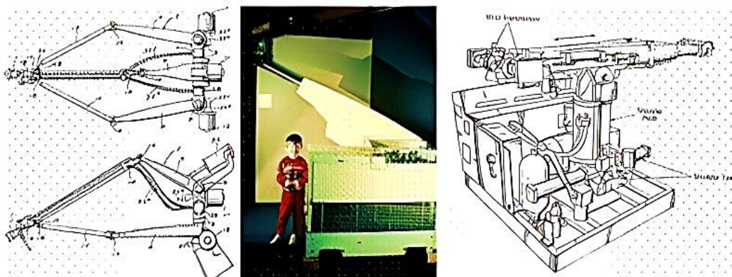
Fig 1. Robotic Arms from the Early 20 th Century: The Pollard Painting Arm (Left) and the Unimate (Right).
