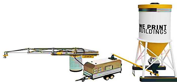
Fig 3. Apis Cor - A 3D Printing Robot Equipped with a Mortar Storage Silo and A Pumping System for Constructing Houses.
