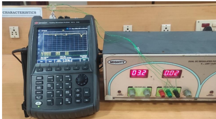
Fig 5. The Reflection Coefficient was Verified with the KEYSIGHT Fieldfox Microwave Analyzer N9917A.
