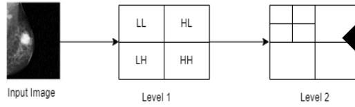
Figure 3 Hierarchical Sub band Technique
