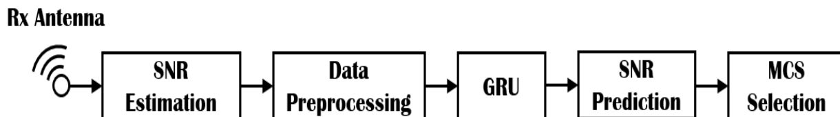
Fig 4. MCS Selection System Block Diagram.
