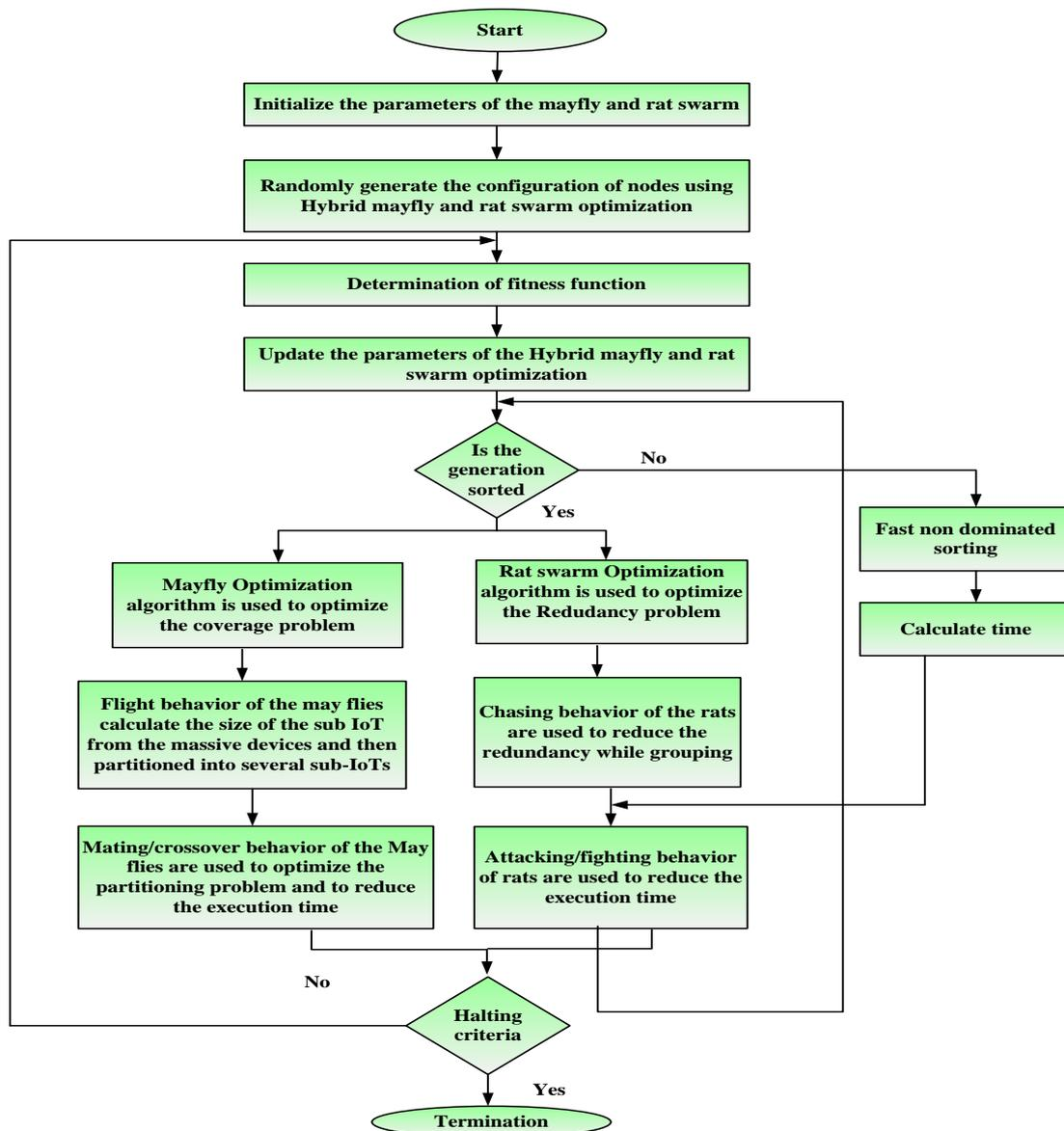
Fig 2. Flowchart for Hybridized Mayfly and Rat Swarm Optimizer algorithm
