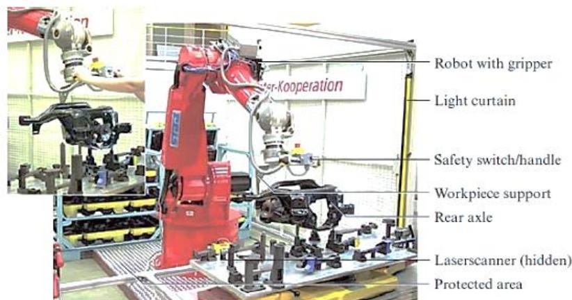
Fig 2. The Collaboration Between Humans and Robots in Order to Carry Out Activities.
