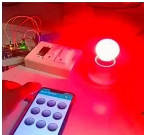
Fig 3. Smart home automation controller using Bluetooth for Android mobile
