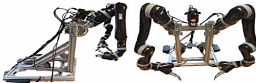
Fig 1. Prototype of a Robot Designed for Harvesting with Two Arms. The First Image Depicts the Lateral Perspective, but the Next One Portrays the Front View.
