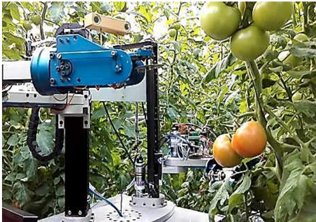
Fig 7. Testing a Dual-Arm Tomato Picking Robot in a Greenhouse.
