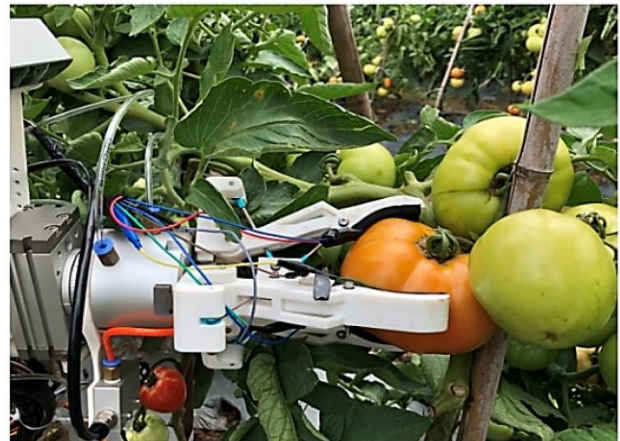
Fig 8. End-Effector for Harvesting Tomatoes using Non-Destructive Pneumatic Clamping Control.
