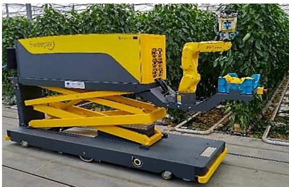
(a) The sweet-pepper-harvesting robot SWEEPER
