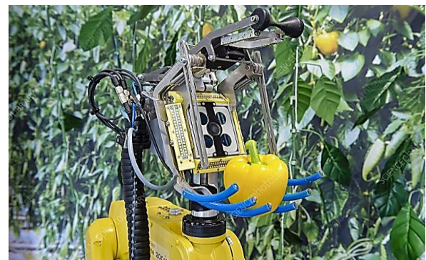
(b) Experimental sweet pepper robot used in the field
