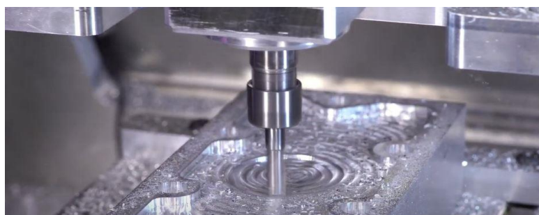
Fig 5. CNC Milling Machine for cutting Aluminium. [Source: https://www.istockphoto.com/photos/cnc-aluminium ].
