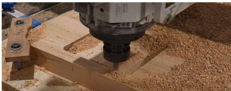
Fig 8. CNC Milling Machine for Cutting Wood. [Source: https://www.istockphoto.com/photos/cnc-wood ].
