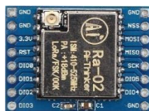
Figure 7: SX1278 LoRa Module
