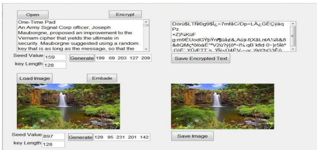
Fig 9. AES- LSB Encryption and Hiding Process.
