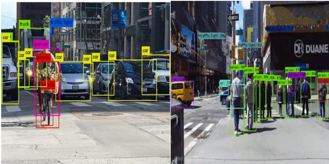
**Fig 4 .** Result of the proposed model from the MOT 20-01 sequence of the real-time MOT 20 dataset.
