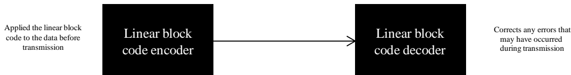
Fig 3. Linear Block Code's Encoding and Decoding Flow
