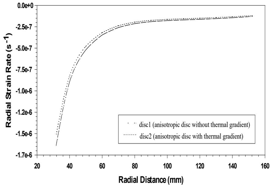
Fig 4. Variation of Radial Strain Rates in Anisotropic Disc With/Without Thermal Gradients.
