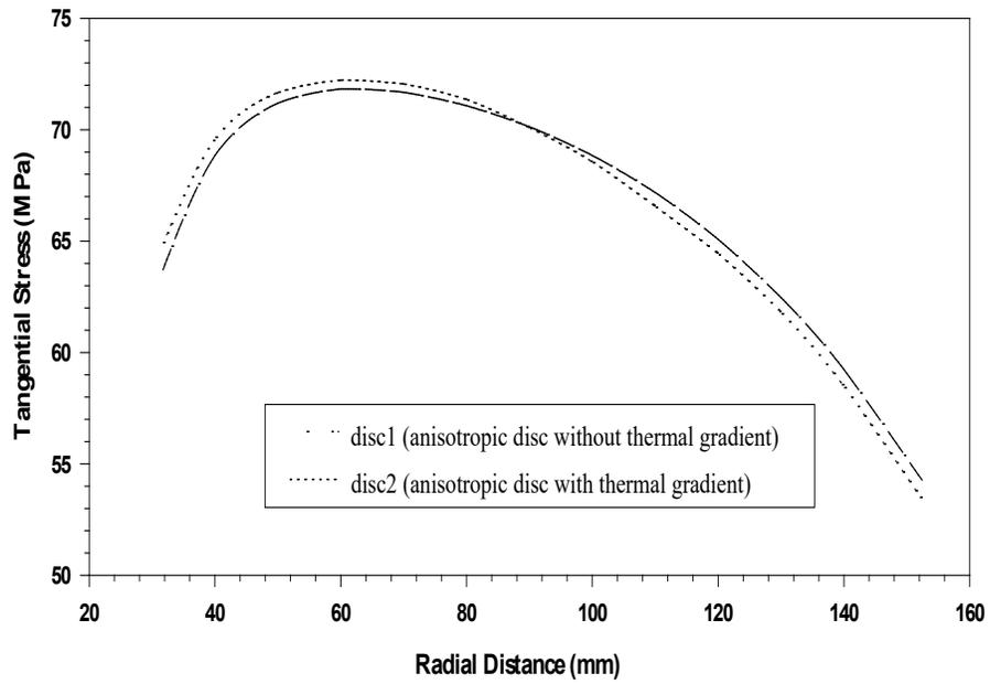
Fig 1. Variation of Tangential Stresses in Anisotropic Disc With/Without Thermal Gradients.
