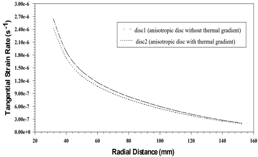
Fig 3. Variation of Tangential Strain Rates in Anisotropic Disc With/Without Thermal Gradients.
