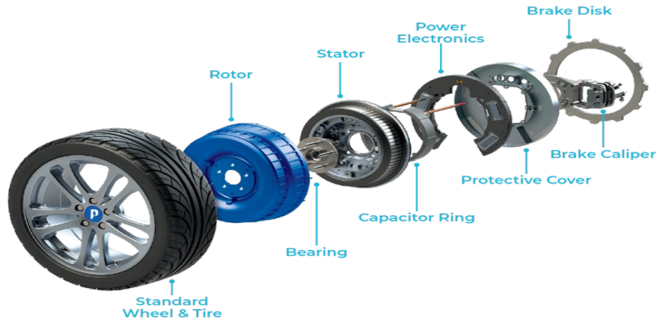
Fig 7. Electric motors to control all wheels.
