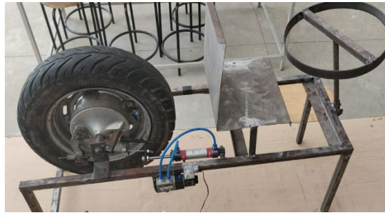
Fig 9. Photograph Of Experimental Setup of Drowsiness Detection and Automatic Braking System.
