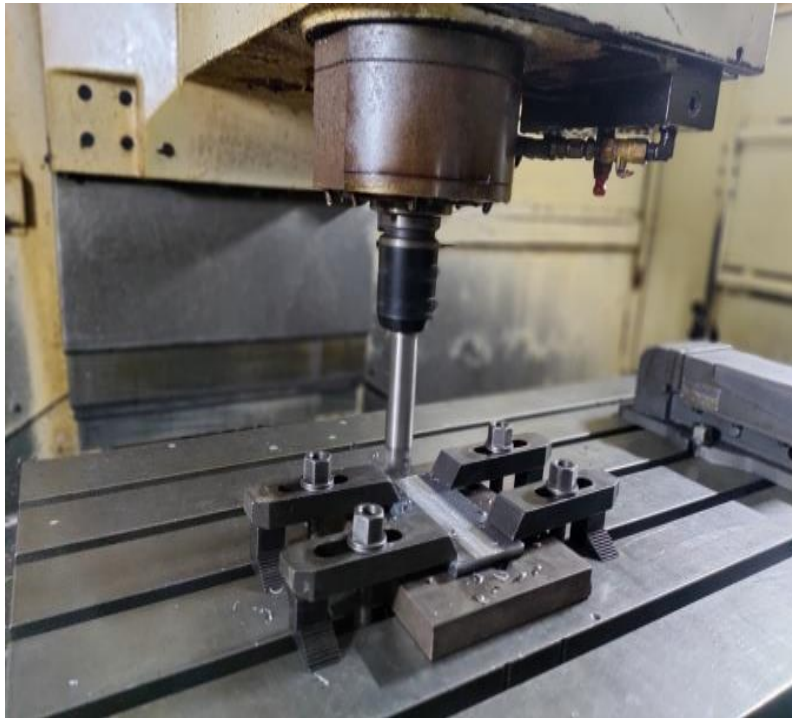
Fig 1. Friction coating process of 314 steel on 1018 steel substrate.
