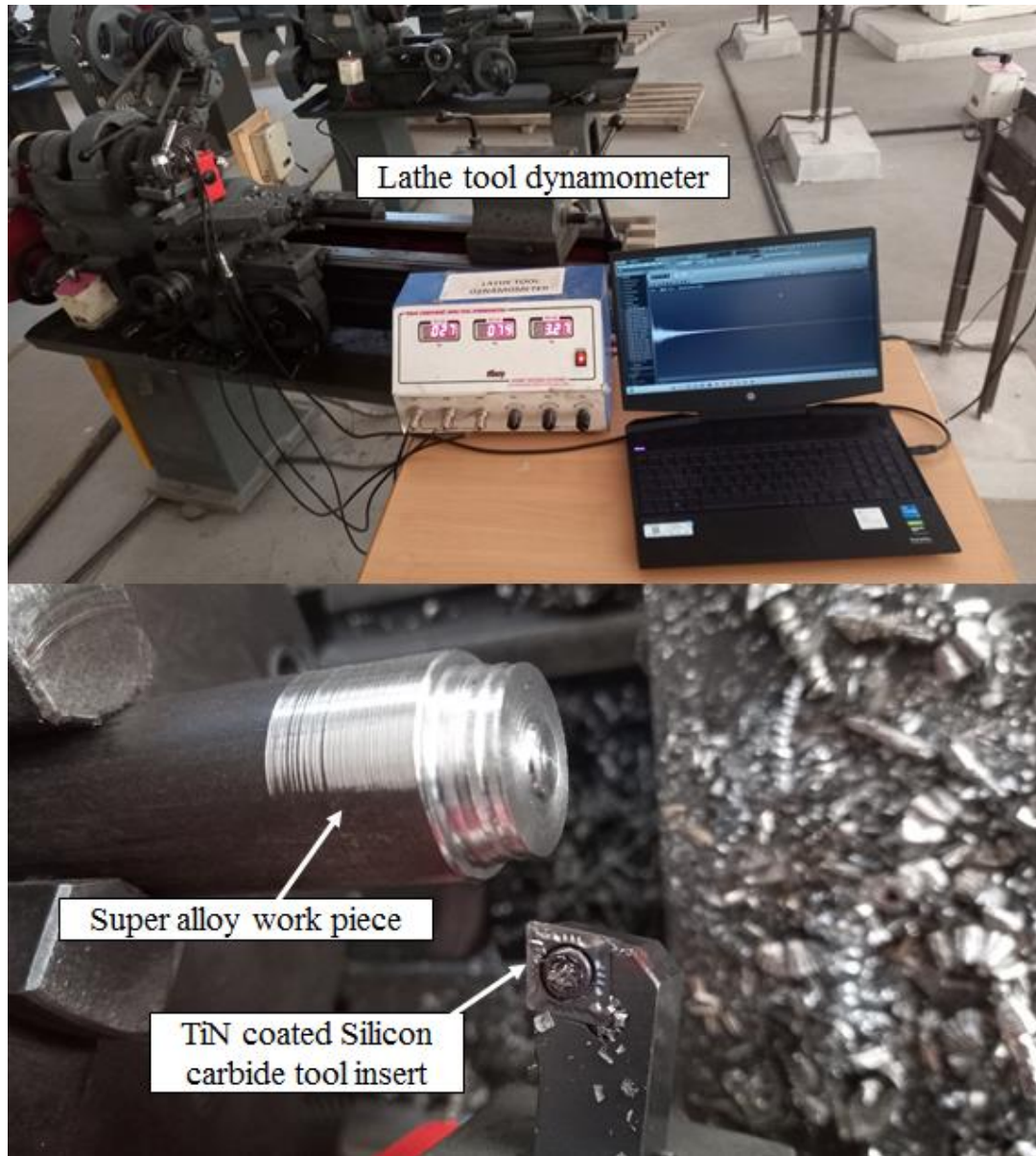
Fig 1. A Typical Experimental Condition for Tool Condition Monitoring in Machining of Super Alloy.
