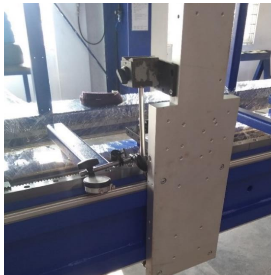
Fig 3. Rack Alignment Using Dial Indicator.
