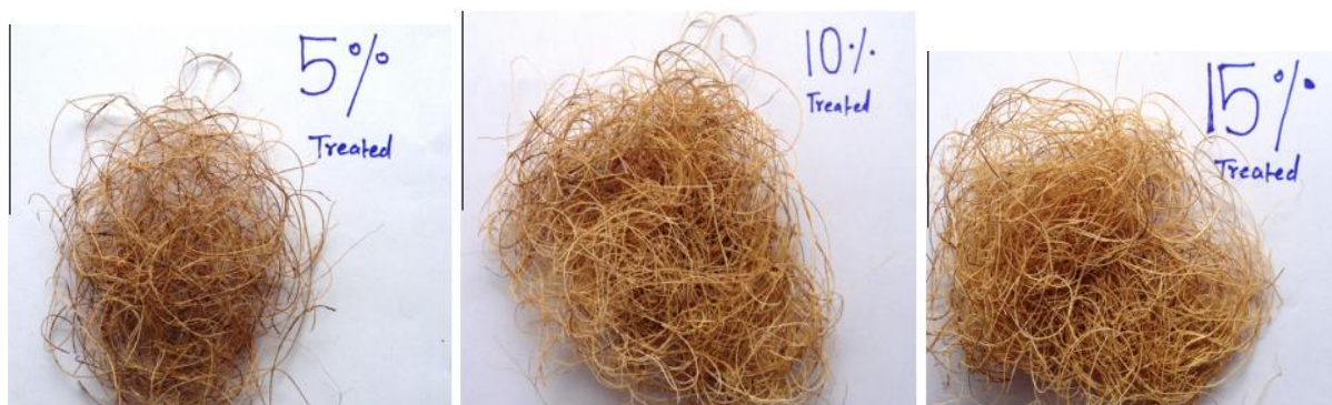
Fig 1. Fiber treated with 5% NaOH, 10% NaOH and 15% NaOH[29]
