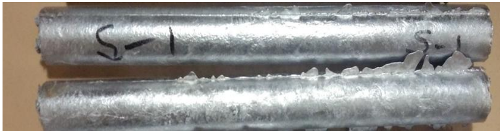
Fig 3. Aluminium Metal Matrix Composites Developed Using Stir Casting Process.
